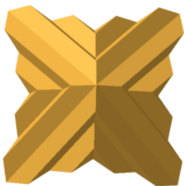
Figure 1: Skew leaf-out folding pattern.
